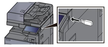
2 When the machine reads the USB drive, "USB Drive is recognized. Displaying files. Are you sure?" may appear. Select [Yes].
