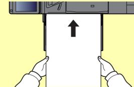
• After printing starts, catch the paper when it is output so that it does not fall. When using the inner tray as the output location, do not stand up the stopper.
