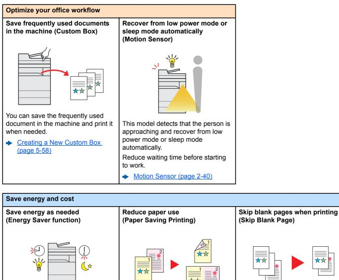
The machine is equipped with Energy Saver function that automatically switched into Low Power Mode or Sleep Mode. You can set appropriate Energy Saver Recovery Level depending on the operation.
