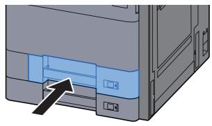
**9** If the optional side feeder is installed, return the side feeder to the original position.
