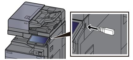
2 When the machine reads the USB drive, "USB Drive is recognized. Displaying files. Are you sure?" may appear. Select [**Yes**] to display the USB Drive screen.
