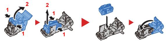
Install the Staple Cartridge Holder (B) or (C).
