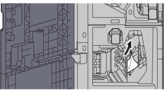
**3** Remove the Staple Cartridge Holder (B) or (C).
