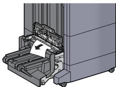
**11** Open the folding unit conveyor guide.
