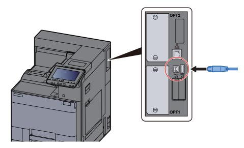
2 Connect the other end of the cable to the PC.
