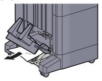
O Press the release lever to pull the folding unit out.
