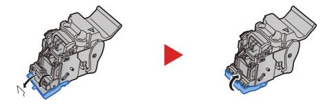
Install the Staple Cartridge Holder (B) or (C).
