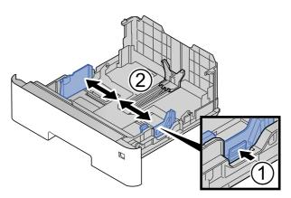
2 Adjust the paper length guide to the paper size required. Press the paper length adjusting tab and slide the guides to the paper size required.
