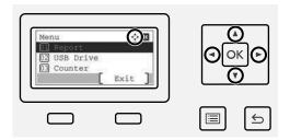
When [OK] is displayed, selecting the [OK] key will confirm the selection. Selecting the [Back] key will return to the previous level in the menu.
