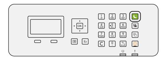
If print data is received during Sleep, the machine automatically wakes up and starts printing.
