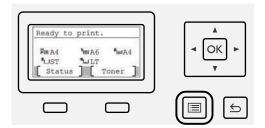
Displays the direction of arrow keys that are useable on the displayed screen.
